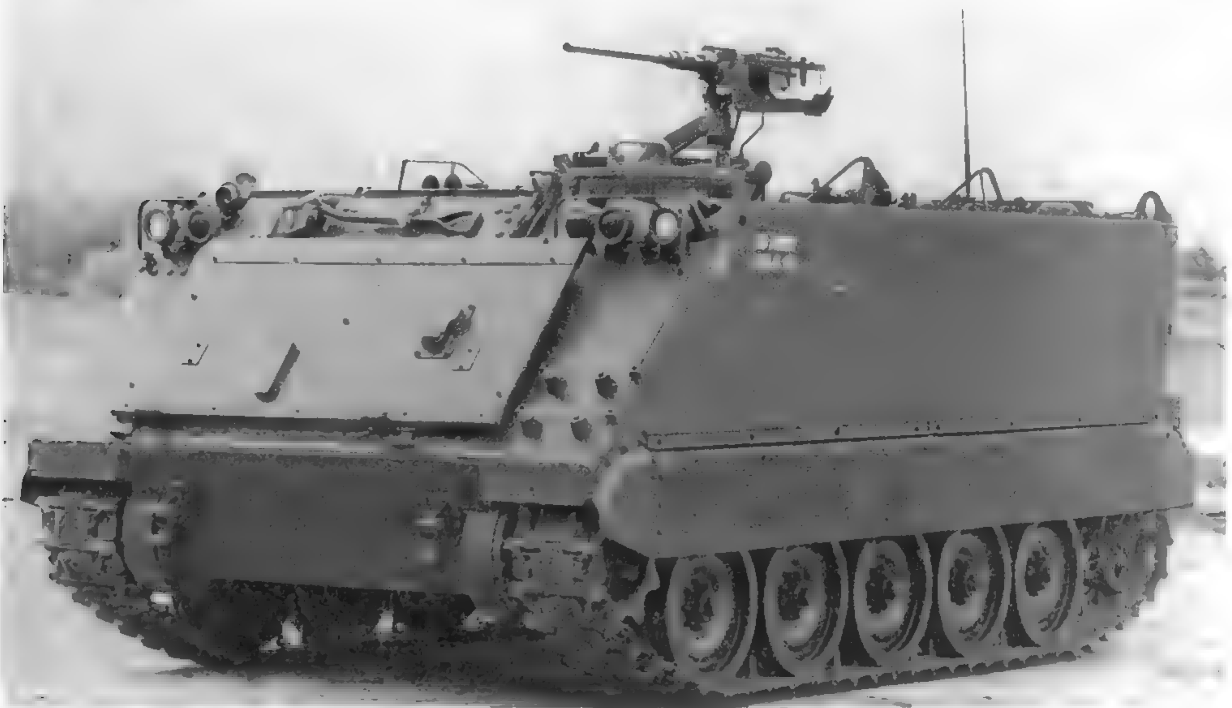
Like the M113, the M113A1 was equipped with a pintle-mounted .50-caliber machine gun. (U.S. Army photo)
